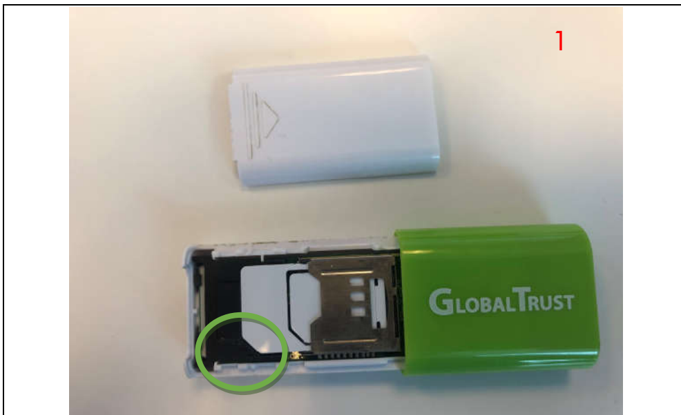
Screen 13: Mini-SIM Format, ACS ACR 101 "c-bird Kombistick"
